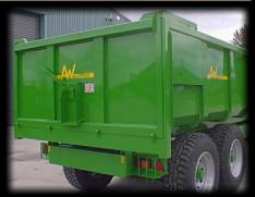
This is fitted with the arms running along the top of the trailer sides and the ram pushing up through the top of the sides. This gives a flush and neat fit but means that the tailboard cannot be used in conjunction with silages sides, extension sides or side to side roll-over sheets.
