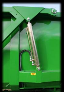
The mounting of the tailboard ram base is kept to a minimum and is tapered
