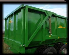
This is fitted with the arms on the outside of the trailer. This gives the trailer a slightly greater over all width but this tailboard can be used in conjunction with silage sides, extension sides and side to side roll-over sheets.
